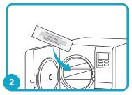
Place **TEST strip** in the center of your sterilizer with a typical load. Do not autoclave mailing envelope.
